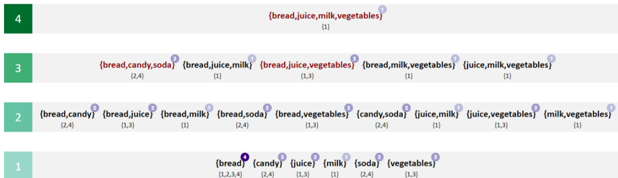
Figure 3.7: The search space of an itemset mining algorithm visualized as a Hasse diagram [48]. The length (i.e., cardinality) is encoded in the vertical position. The support is denoted in purple. The red itemsets occur in the input data.
