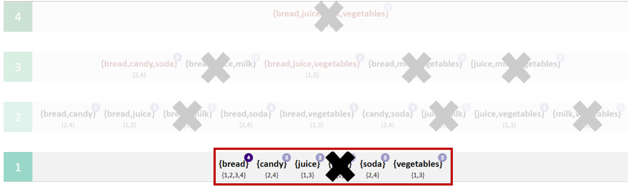
Figure 3.8: The search space is pruned with a minimum support of two (Action 1) depicted by the crossed out itemsets. A second pruning step by length (cardinality) with a parameter setting of the Initial Mining Depth of one drastically reduces the size of the search space (Action 2). The remaining sub-itemsets are highlighted in the red box.
