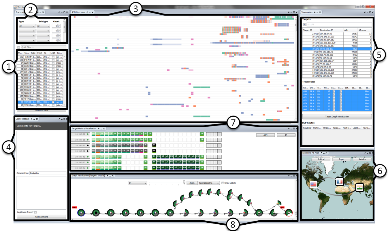
Figure 1: Graphical user interface of the VISTRACER visual analytics tool. (1) and (2) provide access to constraint filters and a table with observed anomalies. (3) Visual ASN Overview with occurred anomalies. A Feedback Panel is provided in (4) and access to individual traceroutes in (5) with map-based (6), glyph-based (7) and graph-based (8) visualizations.
