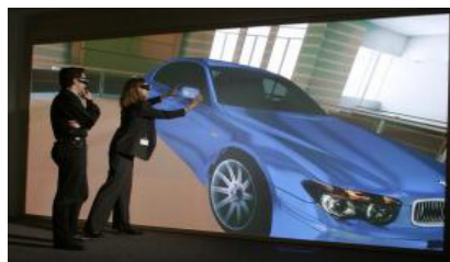
Fig 1: IGD HEyeWall® [1] consisting of a 6x4 array of stereo-projectors (left). Photorealistic interactive rendering on HEyeWall® for industrial design and production, e.g., for the automotive (middle) and garment (right) industries.
