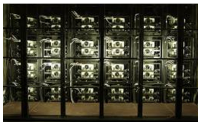
Fig 1: IGD HEyeWall® [1] consisting of a 6x4 array of stereo-projectors (left). Photorealistic interactive rendering on HEyeWall® for industrial design and production, e.g., for the automotive (middle) and garment (right) industries.
