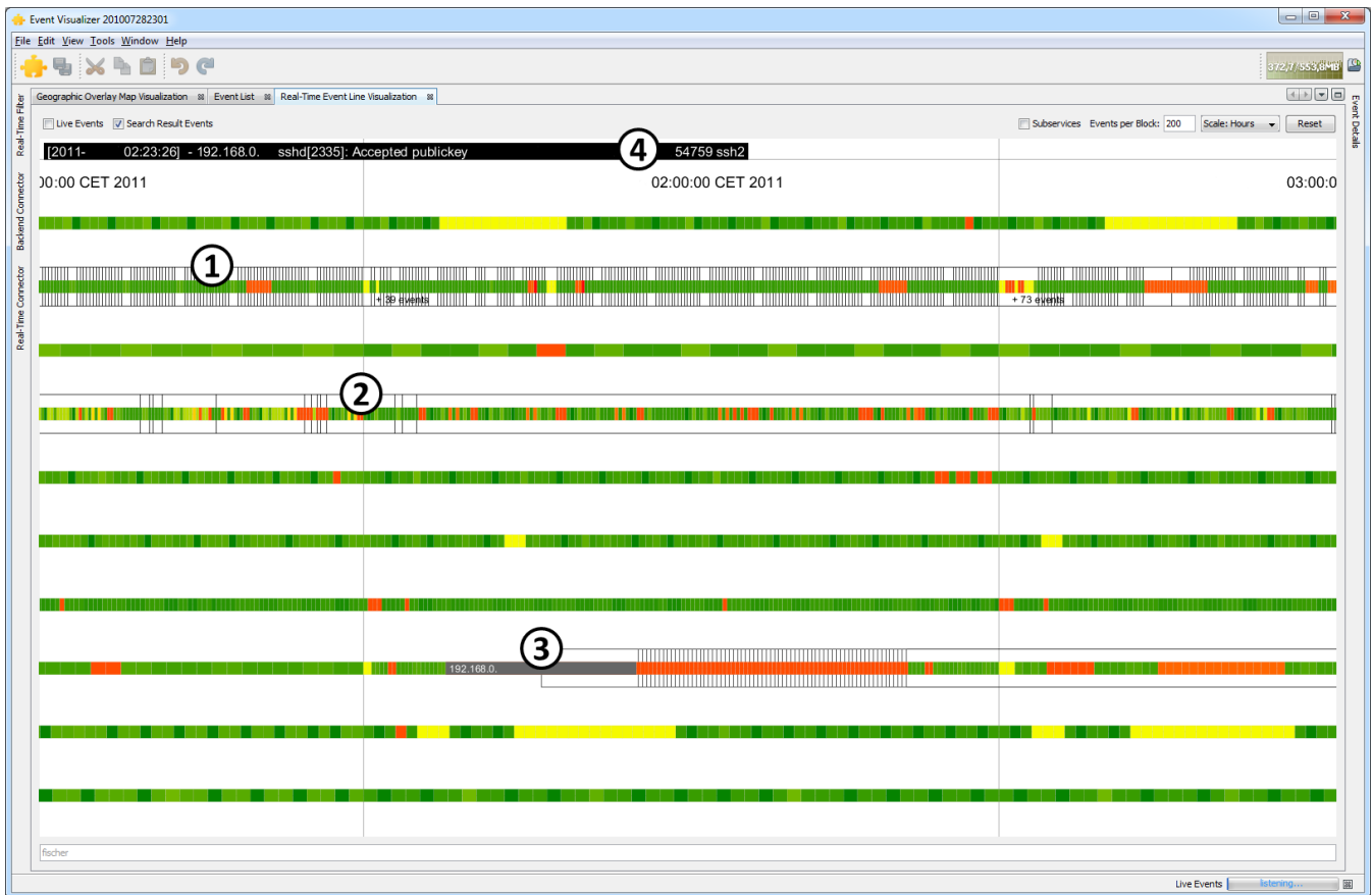
Figure 3: The Relaxed Event Timeline can be used to visually highlight search results (1), which can help to track suspicious user behavior (2) or to notice abnormal patterns (3). Hovering over events provides tooltip information (4).
