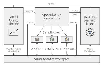
Figure 2: Implementation architecture for Speculative Execution in Visual Analytics. The *Speculative Execution* and *Model Quality Monitor* components can be retrofitted to existing VA systems, together with one or multiple *Model Delta Visualizations*.
