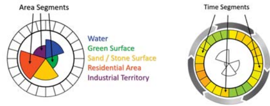
(a) Nightingale glyph: The inner group represents the geographic section of the glyph representation. Every segment indicates the amount of a certain area, that is located within a radius of 1km around a WU station. To the right a colored legend describes the five different area types.
