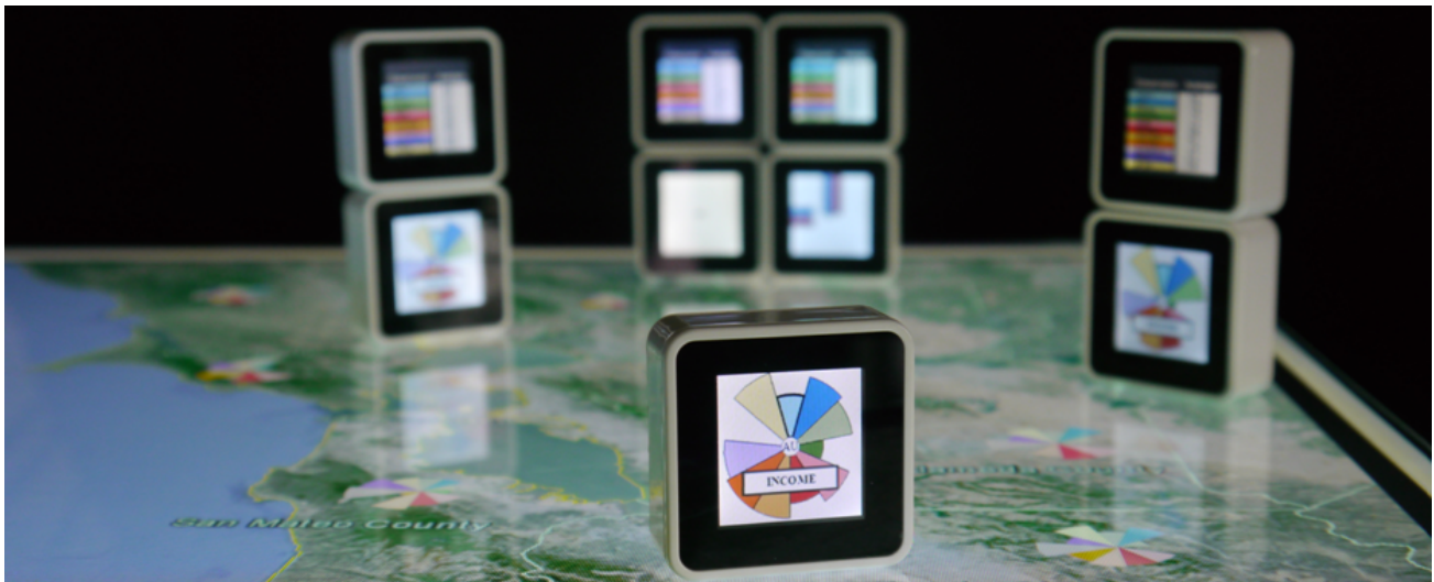
Figure 10. Information Stacking: Example setting of multiple information stacks on top of a multi-touch table. Depending on required granularity, details of data points can be visualized with multiple stacked cubes.
