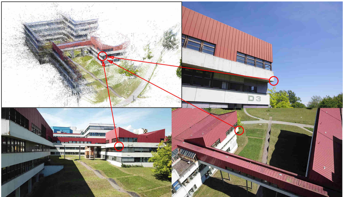
Figure 5.13: Sparse reconstruction (top left), created through Structure-from-Motion approach by matching key-characteristics in different source images - e.g., feature correspondence of pixels in red circle.
