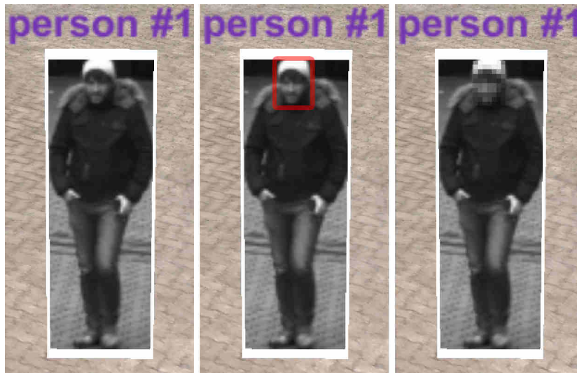
Figure 5.29: Faces of displayed persons within the 4D reconstruction can be anonymized for privacy reasons. A face detection algorithm detects the bounding boxes of faces (center) which are subsequently blurred in the displayed content throughout the visual analysis (right).
