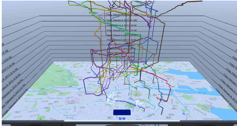
Figure 2.8: A space-time cube is visualized in a virtual reality environment by Wagner et al. [389]. The abstract variable time is mapped to the height of trajectories embedded in the geographic visualization. Image courtesy of Jorge Wagner.
