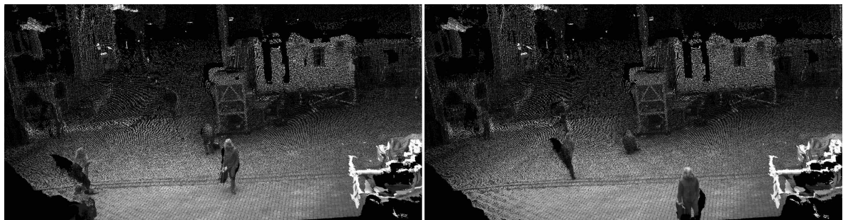
Figure 3.7: Dynamic point cloud visualization. Each frame in the source video is displayed as a 3D point cloud. The 3D video stream can be played or skipped through by using a timeline slider in the interface.
