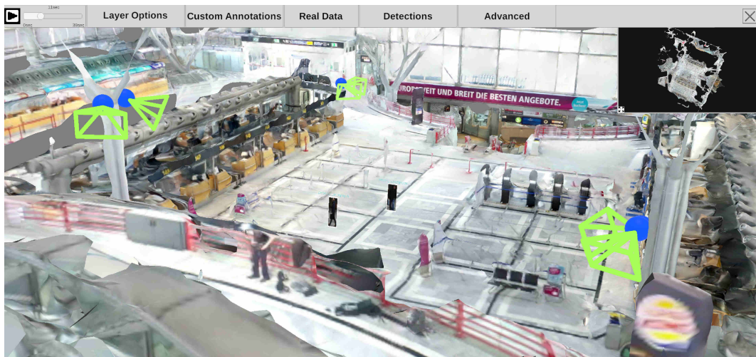
Figure 5.38: Reconstruction of airport in which multiple surveillance cameras are spatially registered. Video streams of the cameras are fed into the system and automatically extracted detections are depicted in the 3D reconstruction in real-time.
