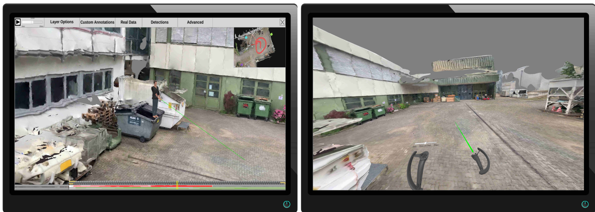
Figure 5.37: Collaborative setup with multiple monitors connected to the system. One monitor shows the usual view of the 4D reconstruction (left) and the other one, a view from the simultaneous observer's perspective in VR (right). An avatar of the VR observer is displayed in the desktop interface (left).
