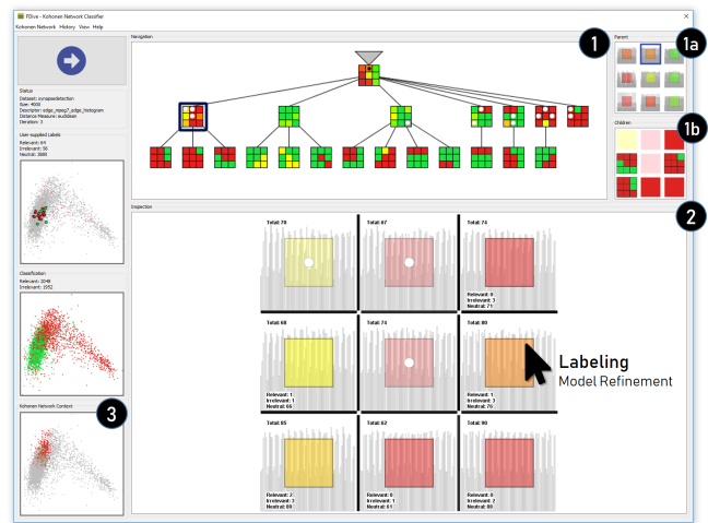
Figure 6: Visual Exploration of SOM Model: 1) Classifier tree. 1a) Parent of the currently observed SOM. 1b) Children of the current SOM. 2) Detailed SOM Display. 3) Scatter plot highlighting data of the SOM node.
