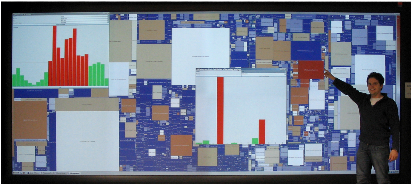
Fig. 5. Hierarchical Network Map displaying all 19 731 autonomous systems (one can still zoom in twice for details) on a large display wall (5.20m \times 2.15m, 8.9 Megapixels, powered by 8 projectors). The query interface on the top left shows the traffic distribution over time and specifies the selected data, in this case the traffic entering the gateway of the University of Konstanz on well-known ports (0-1023) on Nov. 29, 2005 using “transferred bytes” as measure with logarithmic color mapping. One recognizes a heavy traffic load from AS 3320 (red) of “Deutsche Telekom” as well as to neighboring autonomous systems in Germany. A port histogram reveals high activity on the web ports 80 and 443. For security and privacy reasons, the data was aggregated and sanitized.
