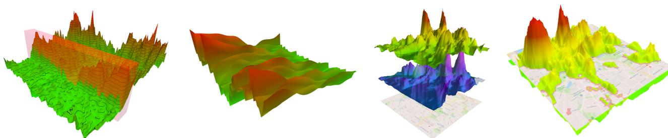
**Figure 1:** Heightmaps in VR. We investigate the design space of VR heightmaps, discuss interaction techniques, such as interactive color adaption, selection (left), and zooming/filtering (center left). The overall focus is set on comparative heightmap visualizations. We use a stacked multi-layer design (center right) and enable the user to interactively position layers of heightmaps (right).
