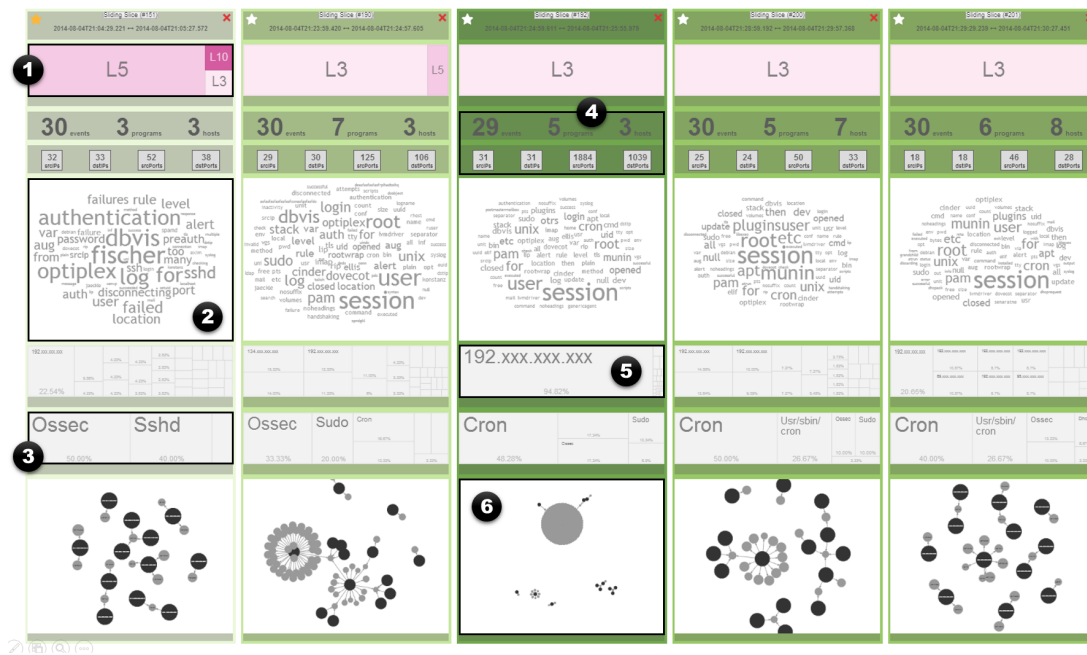
▲ Figure 5.7 — Example of findings using NVisAware . Visualization to monitor data streams using sliding slices to reveal interesting findings. The interactive display can be explored by the analyst while new sliding slices are continuously added. Reprinted from [79]. © 2014 Copyright is held by the owner/author(s). Publication rights licensed to ACM.
