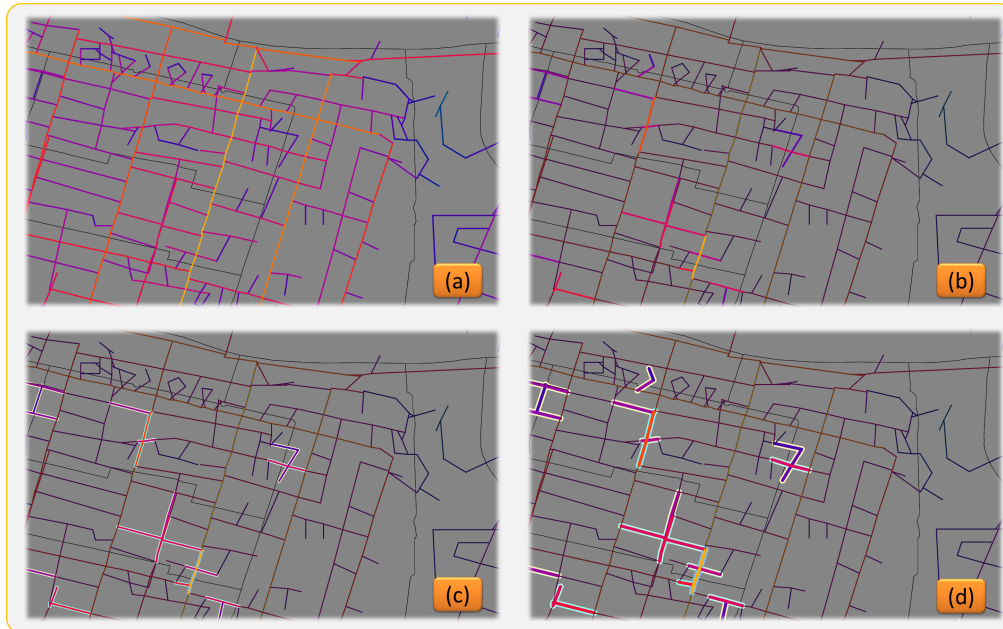
Figure 5.13: Image taken from [18]. Boosting of a high-frequency street-network visualization. The analyst searches for street segments with similar features to a target street, which are boosted by the visualization. (a) No boosting. (b) Boosting with visual attention. (c) Boosting with visual attention and contrast effects. (d) Adapting the width of streets and borders to increase contrast effects exploiting the contrast sensitivity of the human eye.
