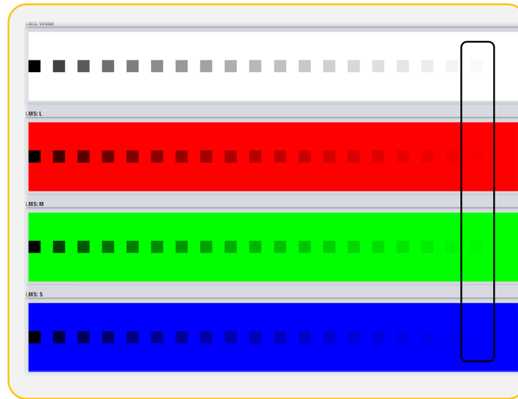
Figure 4.17: The backgrounds share maximum intensity for each RGB channel. The patches on the backgrounds increase linearly in intensity. The user is asked to determine the patch that is just visible from the background, which determines the maximum intensity for each RGB channel that corresponds to the reference white R of the current environment.
