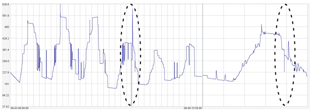
c) Using peak preserving smoothing – peak is preserved and noise removed
