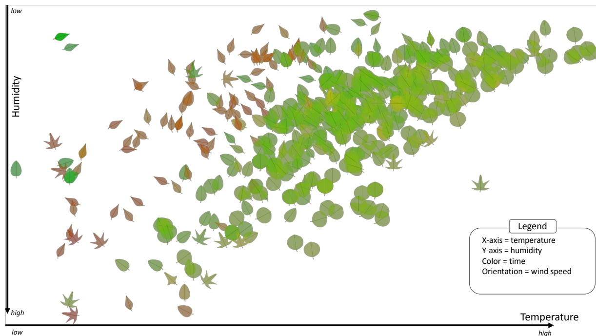
Figure 4.16: Alpha Compositing : Transparency is used to better perceive the data in cluttered areas. Since too many data points are located in the dense regions this aggregation technique does not provide the best view on the data.
