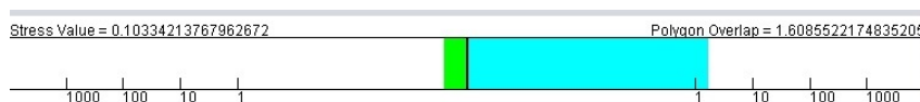
Figure 4.12: Example for visualizing the trade-off between stress and overlap values with horizontal bars. The stress value is exposed to the left in green and the polygon overlap is exposed to the right in blue.
