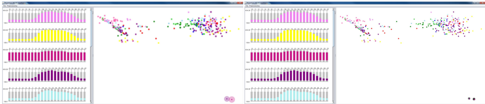
Figure 4.20: Left: Example for a stress value illustration with circle visualization: Bigger circles around the points indicate a higher stress value causation. Right: Example for a stress value illustration with a Gaussian density function: Dense areas that mean high stress value causation are colored in deep black. It is possible to select and deselect dimensions in each visualization on the left side via the bar charts to trigger a recalculation of the projection and the stress value.
