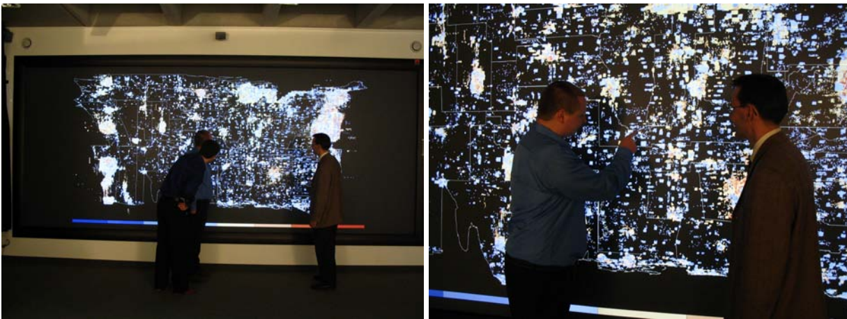
Figure 2.8: High resolution 4 \times 2 Barco DLP based projector ( \approx 9 \cdot 10^6 pixels) i-wall at the University of Konstanz
