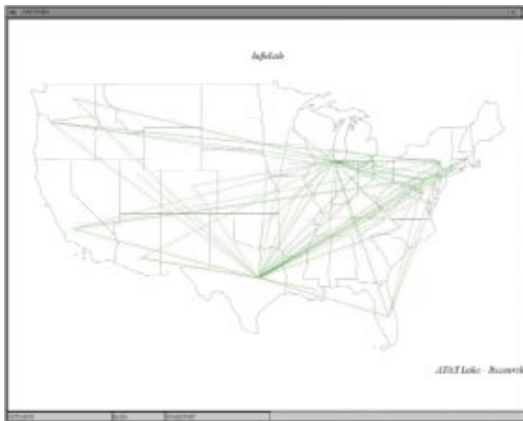
4 Virtual network configuration created by a customer. The display was made by joining network topology and customer-configuration databases.
