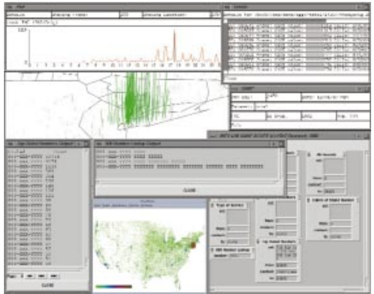
3 Inspection of a network event's impact on customers of a toll-free call center. The display shows the effects of a certain event on geographic locations and originating and terminating numbers.
