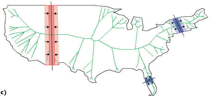
3 Cartogram algorithm: (a) map with area error and medial axis, (b) stretching and contracting the global polygon, and (c) example cutting lines.
